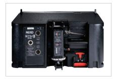
Innovative PistonRig™ and REDLock™ rigging enables any size of system to be flown safely by one person. PistonRig™ allows pre-setting of inter-cabinet angle values. REDLock™ handle locks front rigging points from rear of cabinet. All adjustments made from one position at rear of cluster.
